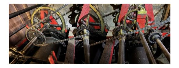
The main issue is that most of the top of the case is missing, and during cleaning work in the tower when the tenor bell was rehung, a large amount of dust and dirt has dropped into the case and into the clock.
