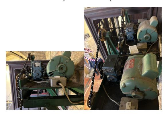
We would suggest that the best course of action for the clock movement is for it to be stripped and thoroughly cleaned on-site, this would also allow all the bearings to be checked for wear & working surfaces polished. Given the lack of serious wear, and the fact that the clock is still running.
