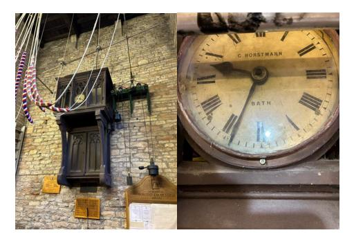
Between the glazed front doors is round glazed aperture showing the setting dial. This is much larger than usual and acts as a time indicator for the ringers, therefore runs clockwise and has its own motion work driven from the centre arbor. This indicates that the clock was supplied by G. Horstmann of Bath – presumably this was the forerunner of the Horstmann Gear Company of Bath who were makers of mechanical time switches.
