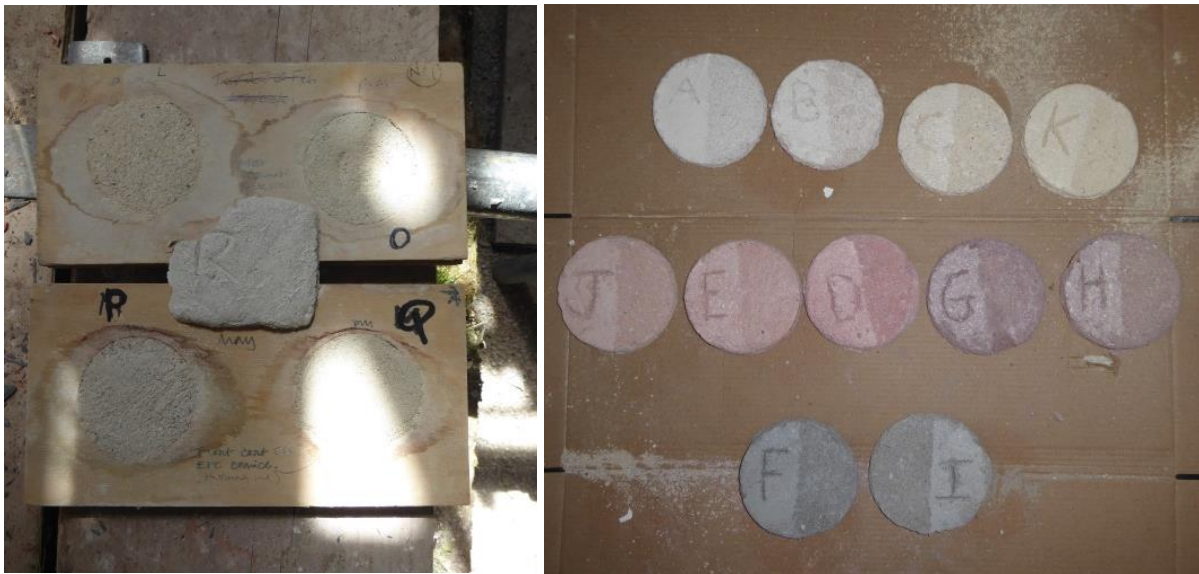
Figure 33 Mortar trials for repointing and mortar repairs
