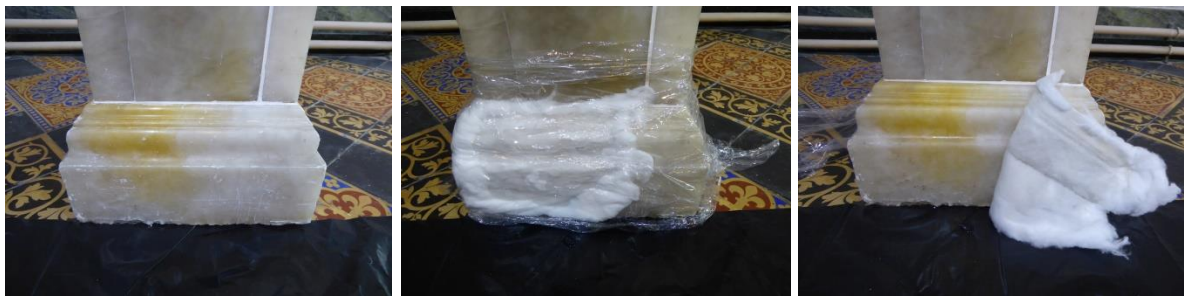
Figure 24 Trials to reduce the ferrous stains to the alabaster surface
