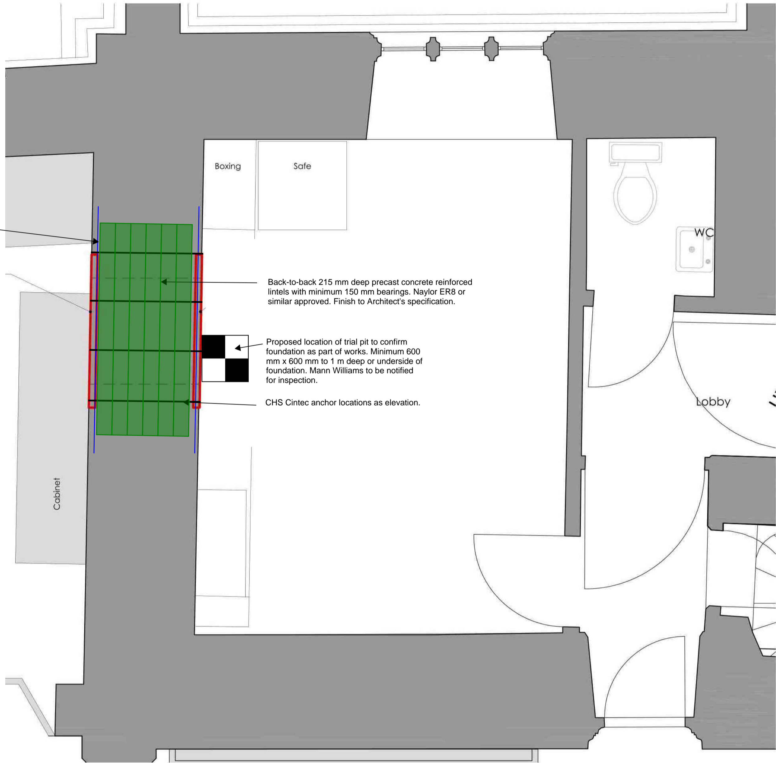
Ground floor plan on proposed opening 1:20
