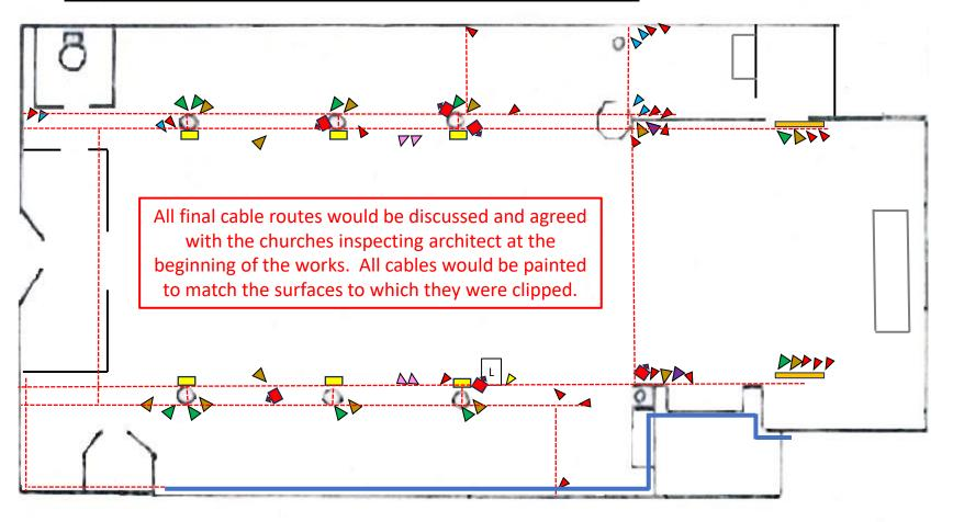
A new 60 Amp supply cable from the external plant room to supply a new distribution board position would be taken under the floor of the South aisle
