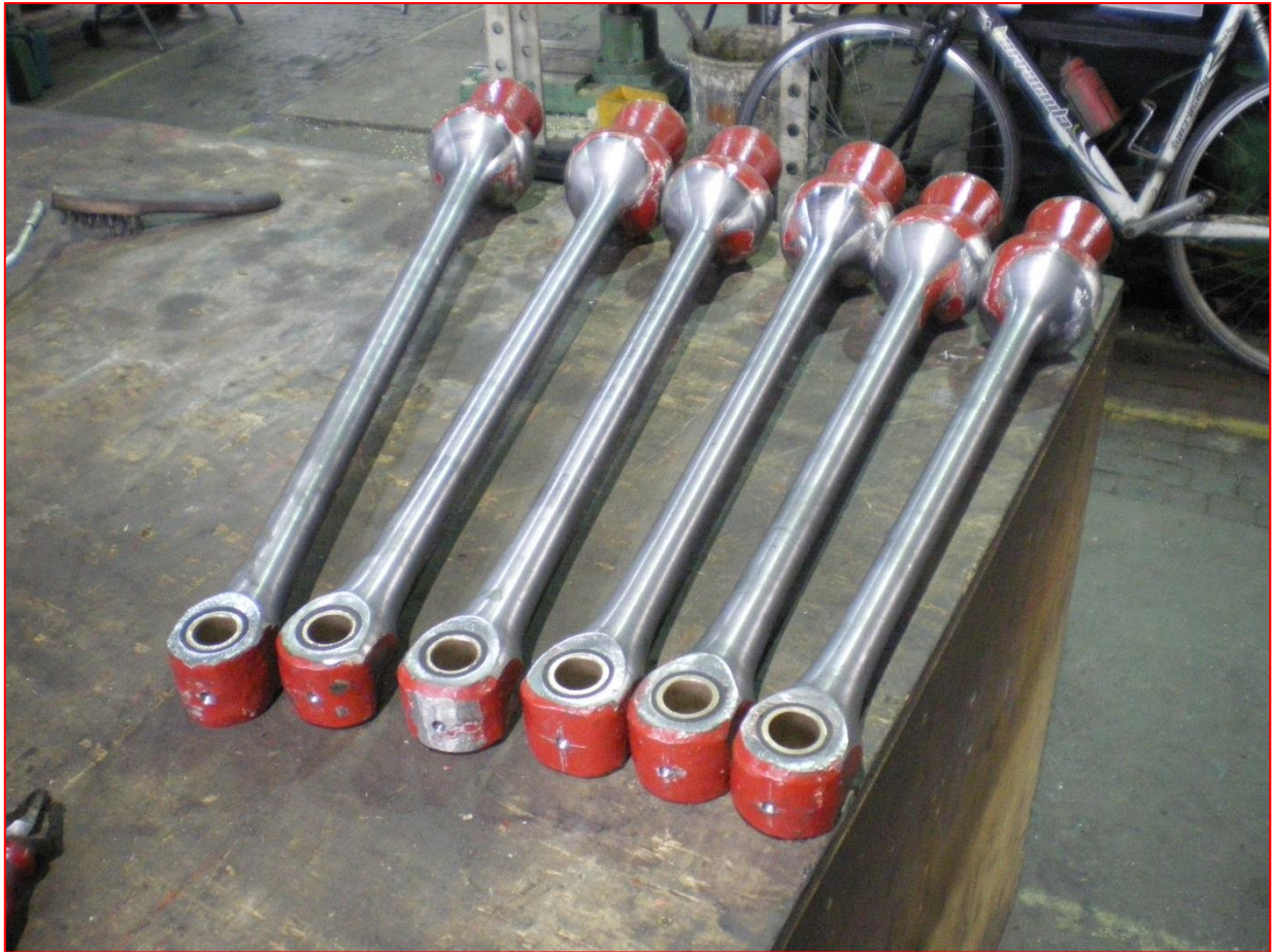
Photo: SG iron clappers with their shafts lathe machined to improve their timing
