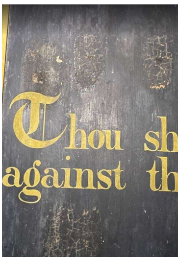
Figure 33 Natural wood knots are located all over the surface, they appear like a large crusty lumps.
