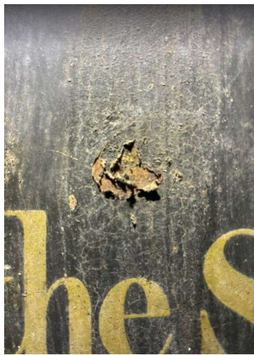
Figure 27 A knot showing the damage made by a sap pocket.
