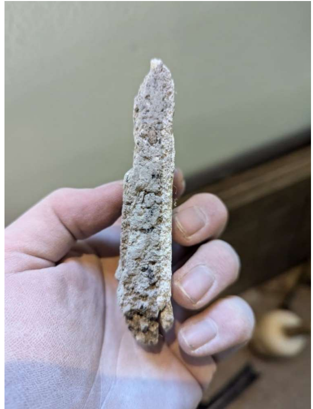
Figure 15 Fragment of two-coat plaster removed
