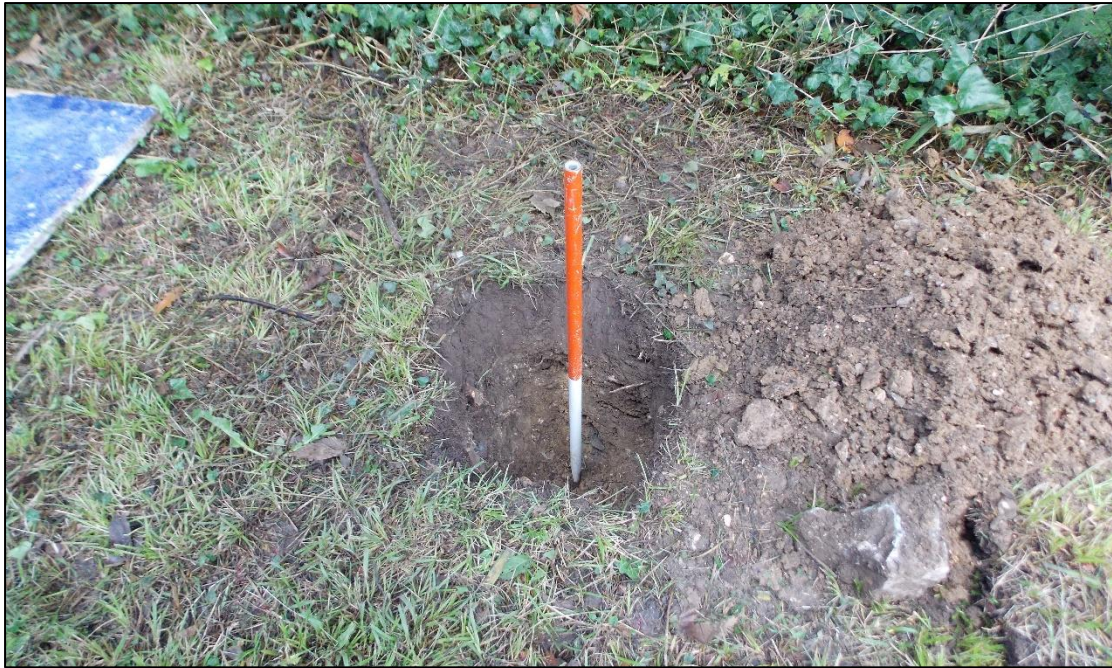
Figure 11. East percolation test hole: facing N, 1m scale.
