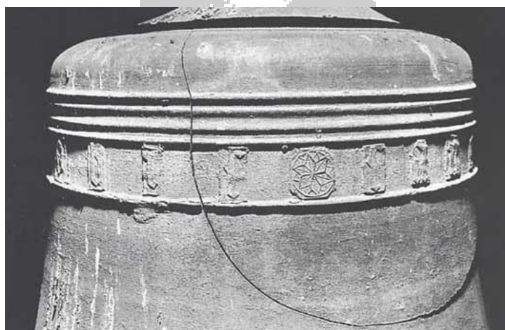
A typical crack caused by corroded cast-in crown staple. (Sparkford, Somerset – Photo Christopher J N Dalton).
