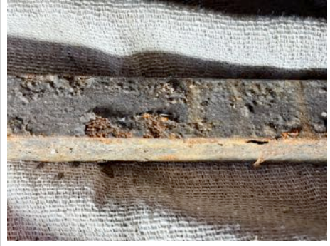
x 50 Magnification Forge coat and the original paint coating layers
