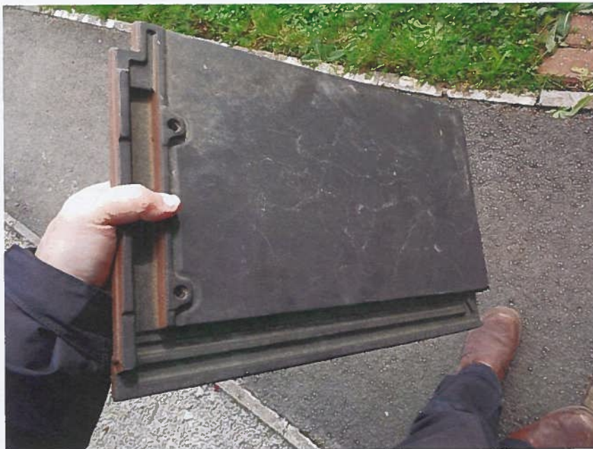
View of Planum interlocking clay tile
