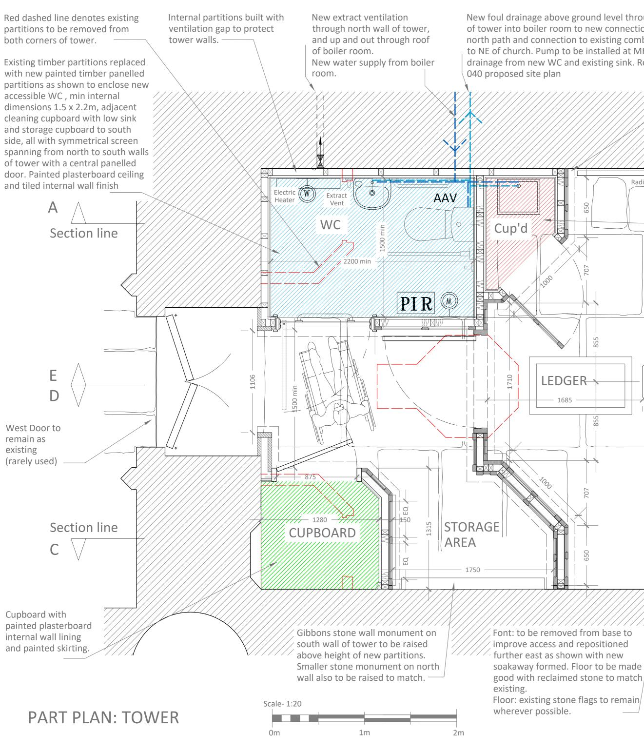
New foul drainage above ground level through north wall of tower into boiler room to new connections beneath north path and connection to existing combined drainage to NE of church. Pump to be installed at MH1 to aid drainage from new WC and existing sink. Refer to drwg  $\mathbf{\Omega}$
