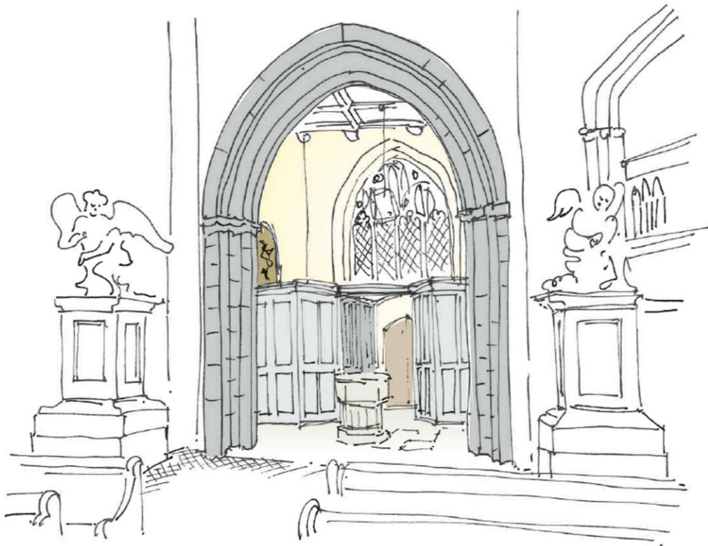
Fig 9: Sketch view of Option 3 seen from the nave. The central doors within the new screen are shown in the open position, with the west door visible beyond
