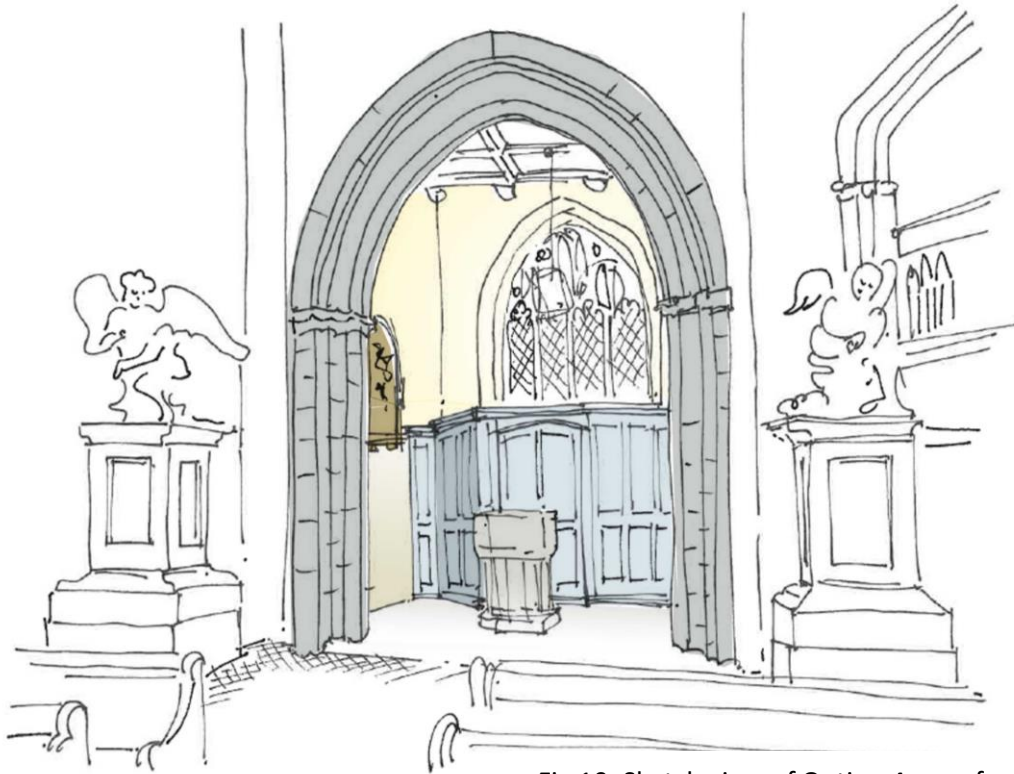
Fig 10: Sketch view of Option 4 seen from the nave. The central door within the new screen is shown in the closed position, and the stone monument on the south wall is visible.
