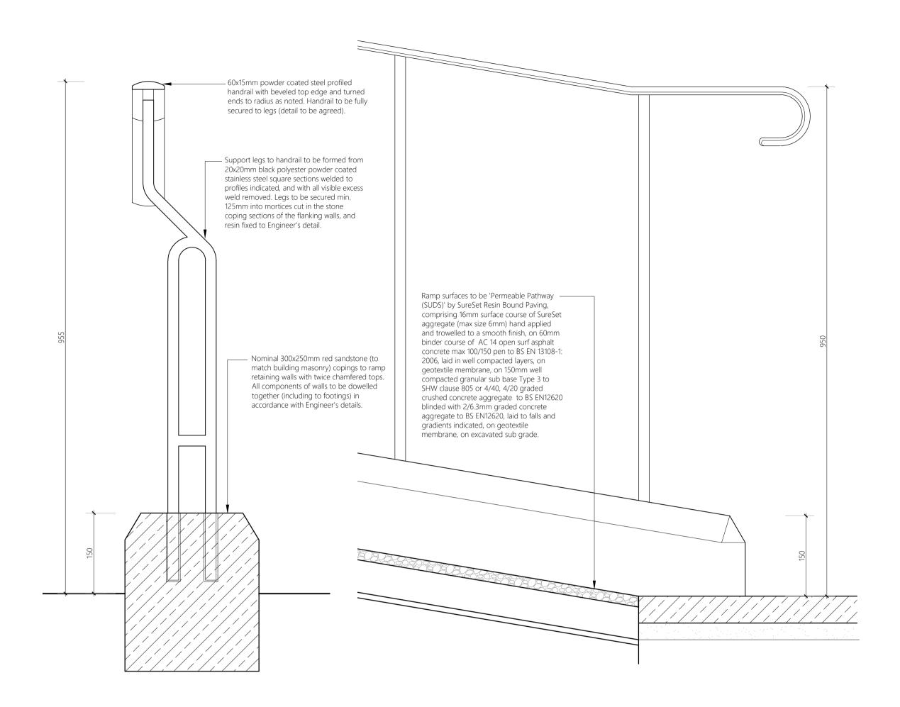
Section Through Ramp's Kerb & Handrail Scale 1:5
