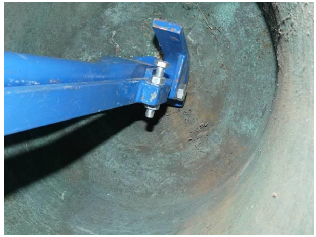
The new electromagnetic hammer units mounted firmly on the outside of the bells
