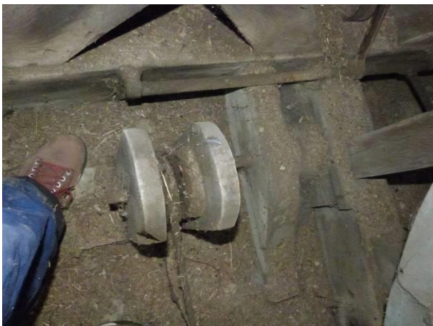
The old rope pulleys left in situ and the new pulleys for the lever safety clappers mounted on the floor. These pulleys are from the Bartol range design for marine usage.
