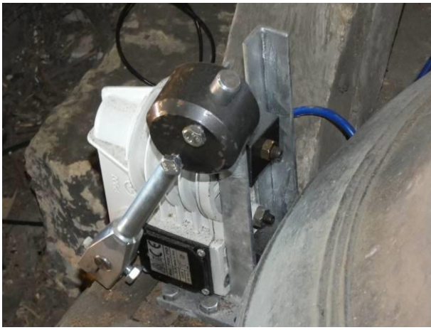
The new electromagnetic hammer units mounted firmly on the outside of the bells
