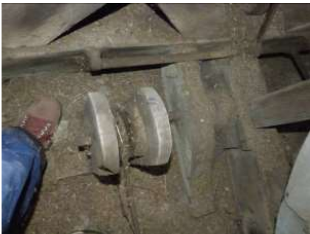
The old rope pulleys left in situ and the new pulleys for the lever safety clappers mounted on the floor. These pulleys are from the Bartol range designed for marine usage.
