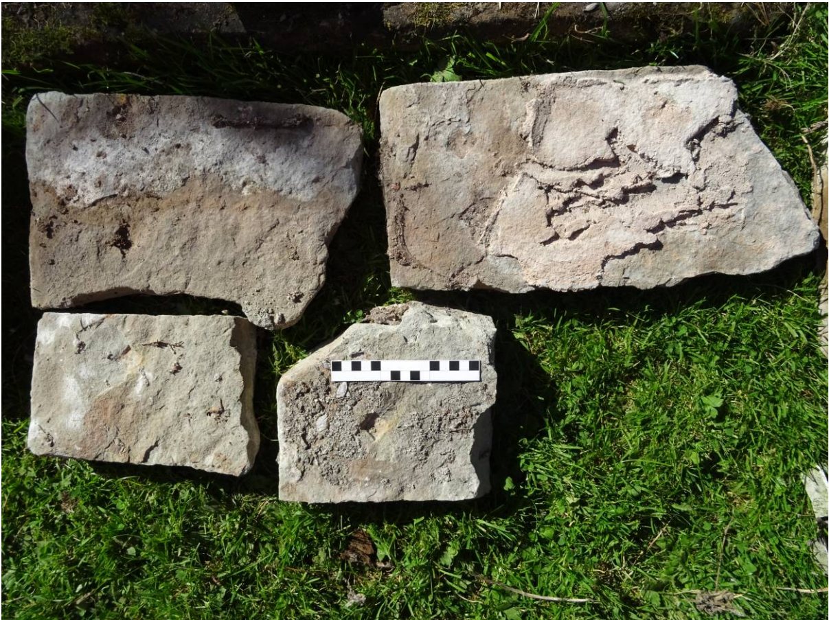
Plate 25. A selection of the rubble infill from the core of the monument
