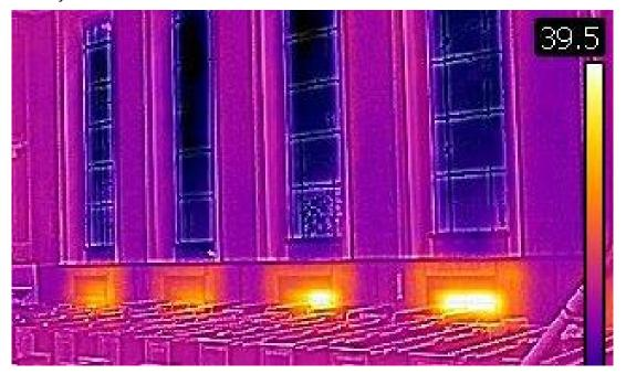
Above (L), radiator in chancel, operating well. Above (R), radiator fitted with two pairs of fans, which are exporting the heat more efficiently and drawing air
