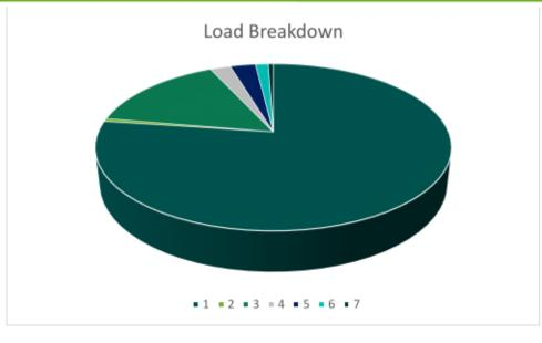
KEY 1 Gas Heating 2 Electric Heating 3 Lighting internal 4 Lighting external
