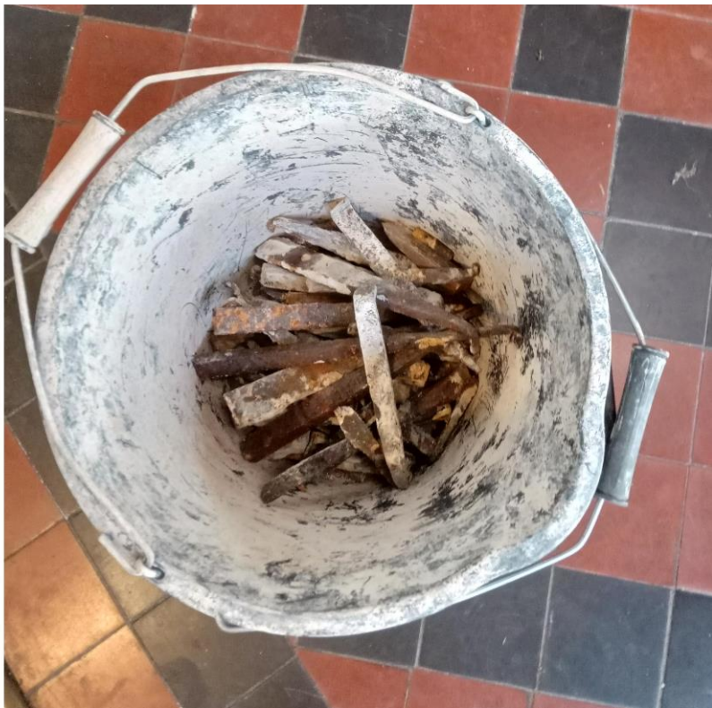
Left: Rusted ferrous fixings removed from the monuments
