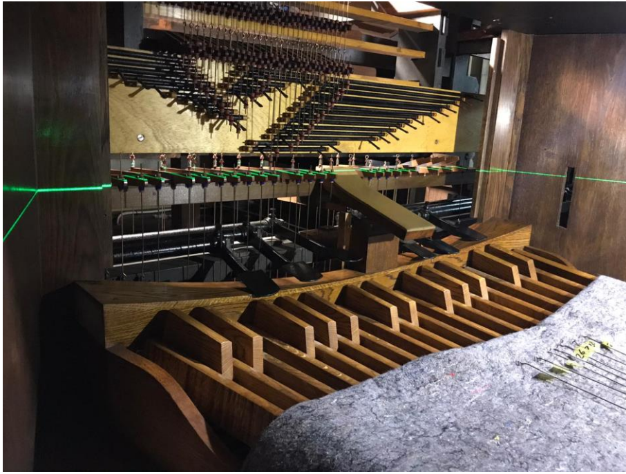
Regulating restored mechanical action using laser sights
