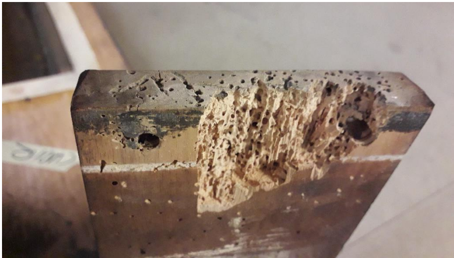
Drawstop action register destroyed by woodworm
