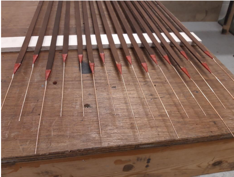
New phosphor bronze wires whipped in original style
