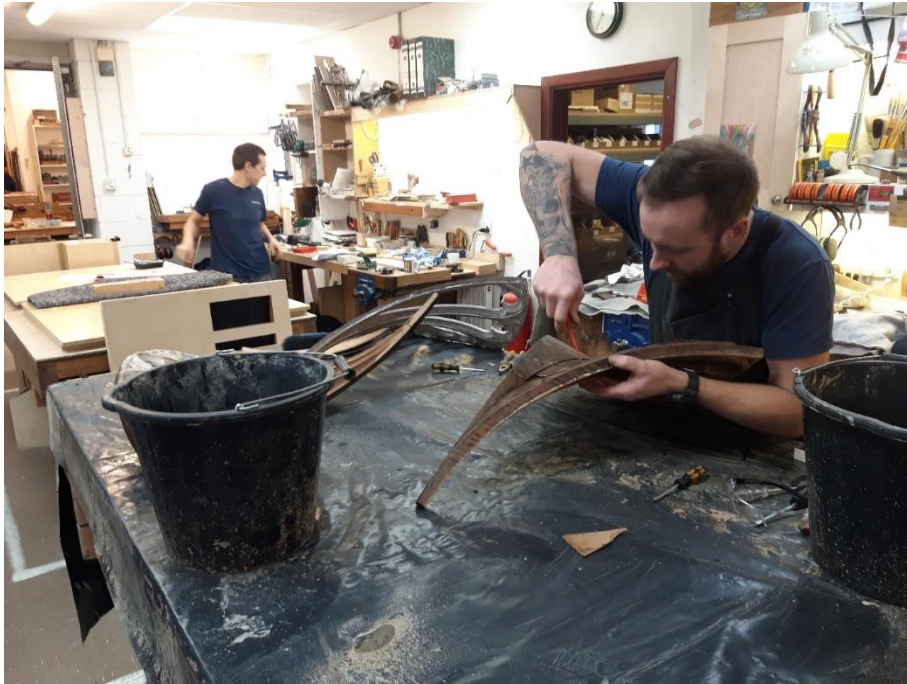
Cleaning off the liming with a stiff brush and warm water
