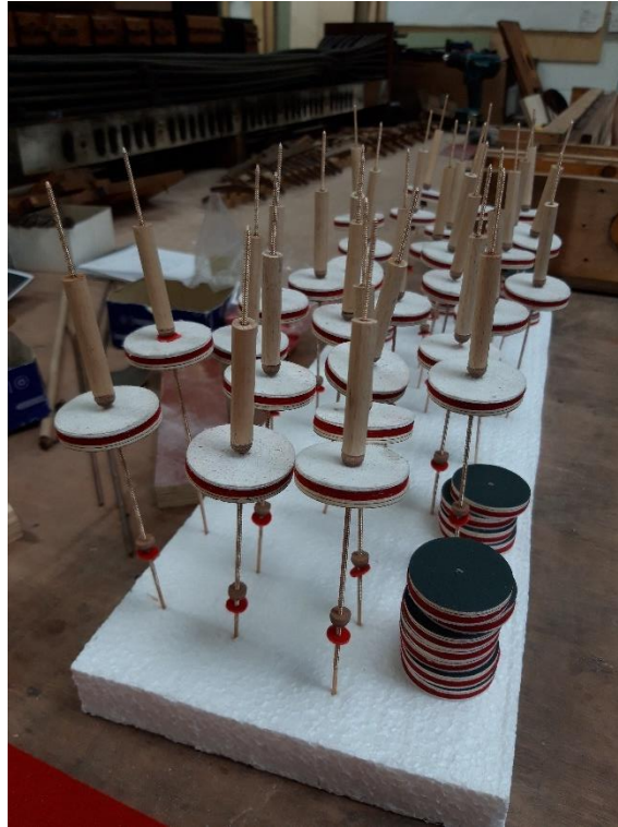
New valve coverings
