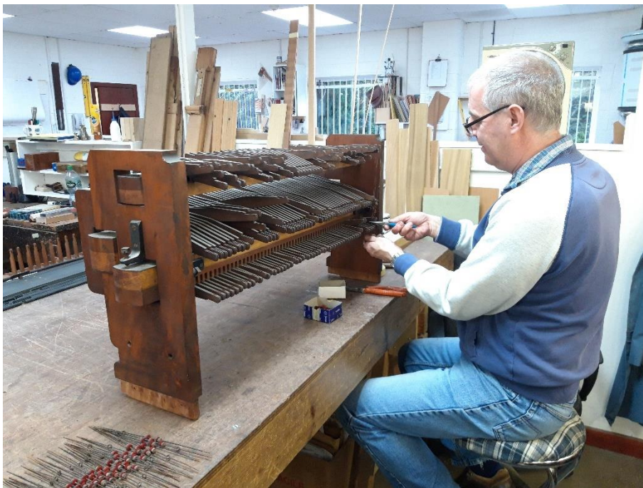
Restoration of coupling chassis
