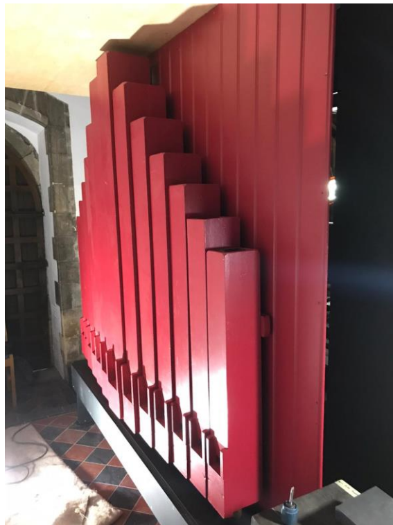
New casework panelling at rear of instrument, and relocated Open Diapason 16' pipes that had previously been attached to the right-hand elevation of the case as per below
