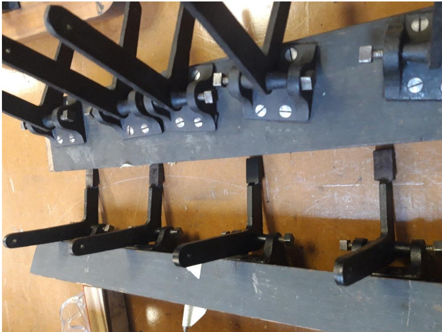
Drawstop squares, including one we had to make new due to the original being missing
