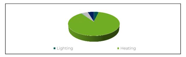
As can been seen from this data, the heating makes up by far the largest proportion of the energy usage on site. The lighting load is small due to adoption of low energy lighting for most internal fittings.
