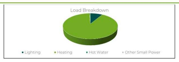
As can been seen from this data, the heating makes up by far the largest proportion of the energy usage on site. The other significant load is lighting.
