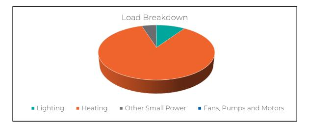
As can been seen from this data, the heating makes up by far the largest proportion of the energy usage on site. The other significant load is lighting.
