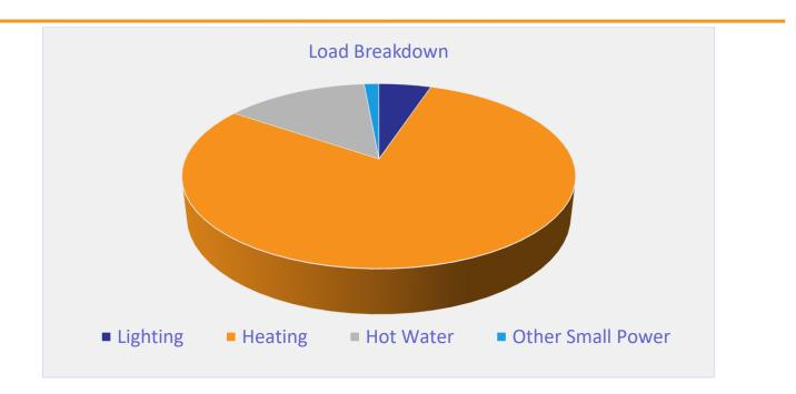
As can been seen from this data, the heating makes up by far the largest proportion of the energy usage on site. The other significant load is hot water.
