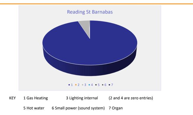
As can been seen from this data, the heating makes up by far the largest proportion of the energy usage. The lighting load is significant as other items of electrical equipment are of low power and/or used infrequently. This graph does not take into account the recent use of electrical heating (six portable heaters of total load 12.4kW which were not in use during the billing period)
