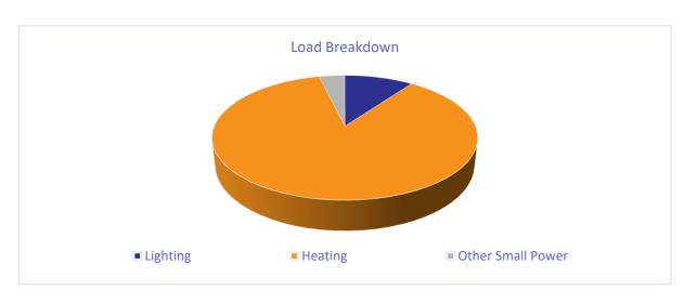
As can been seen from this data, the heating makes up by far the largest proportion of the energy usage on site. The other significant load is lighting.
