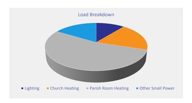
As can been seen from this data, the night storage heating to the parish rooms makes up by far the largest proportion of the energy usage on site.
