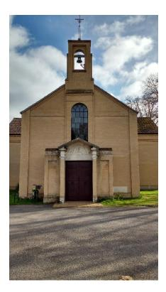
The doors are firmly closed, but much thinner than the walls so are allowing heat to escape by radiation. This shows the importance of having a draught lobby inside.
