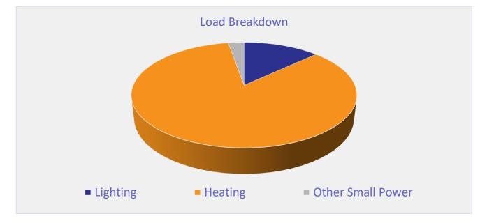
As can been seen from this data, the heating makes up by far the largest proportion of the energy usage on site. The other significant load is lighting.
