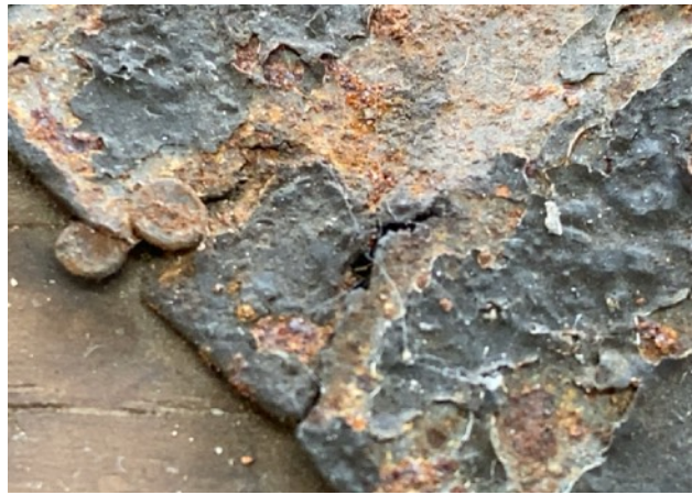
Detail of the surface of the heart showing the lifting paint, rust spots and small iron nails.
