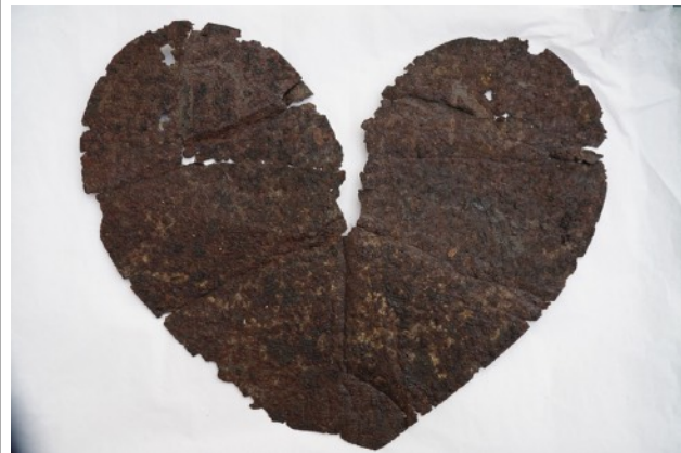
The iron heart after cleaning and during the process of consolidation with the Paranoid B67.
