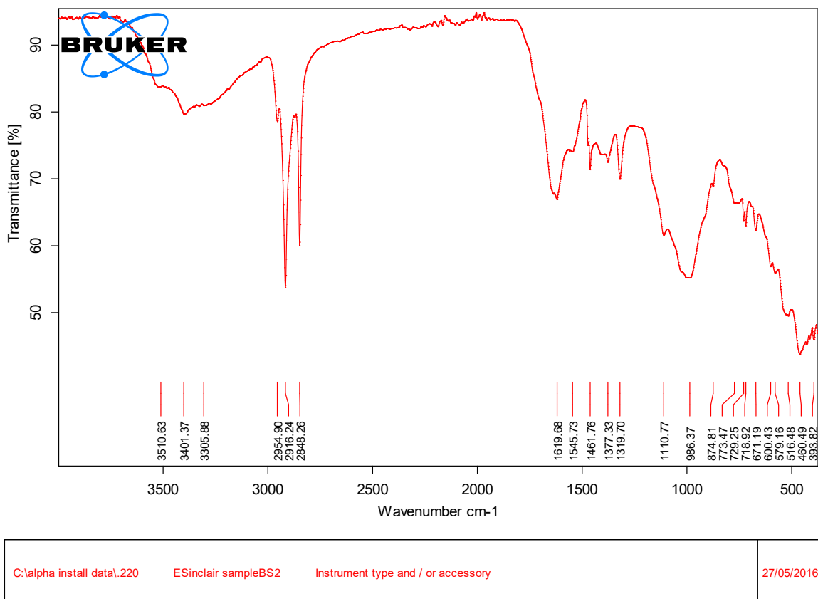
Figure 1 FTIR Spectrum of sample BS2 white bloom side of paint chip
