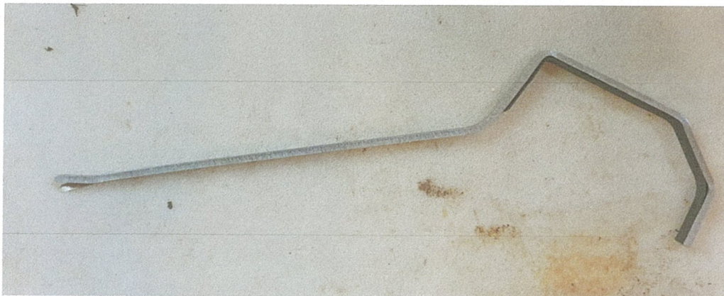
Plate 13: detail of one of the shaped restraining cramps for fragment 3
