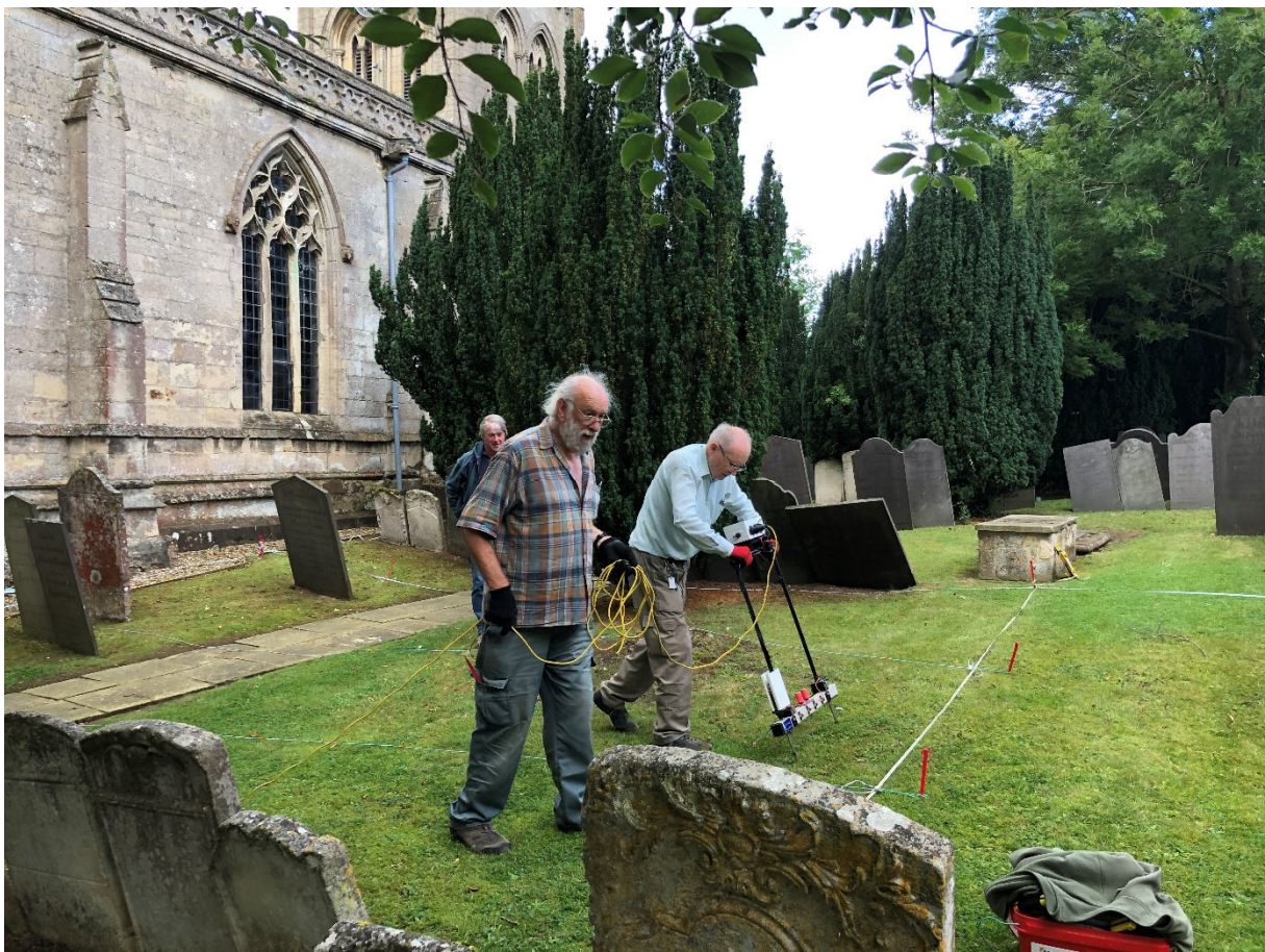
Figure 10: Resistivity survey being undertaken. The entrance to the crypt is visible in the top image.
