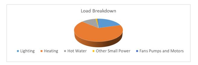
As can been seen from this data, the heating makes up by far the largest proportion of the energy usage on site. The other significant load is lighting.
