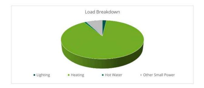
As can be seen from this data, the heating makes up by far the largest proportion of the energy usage on site. The other significant load is other small power.
