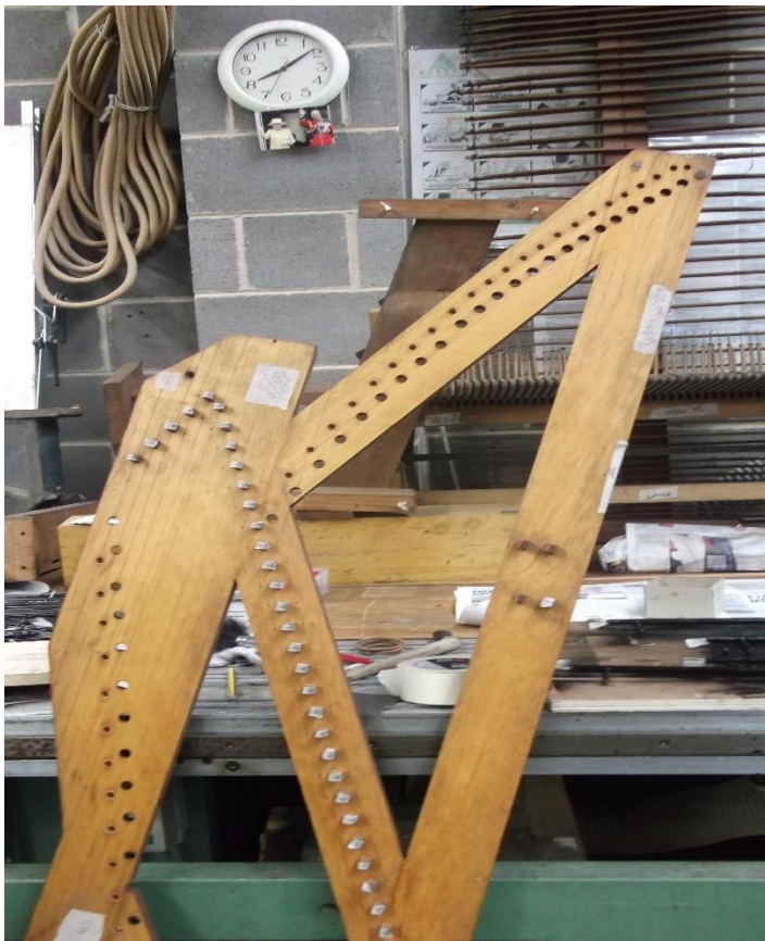
The roller-board frames with studs removed for re-bushing.
