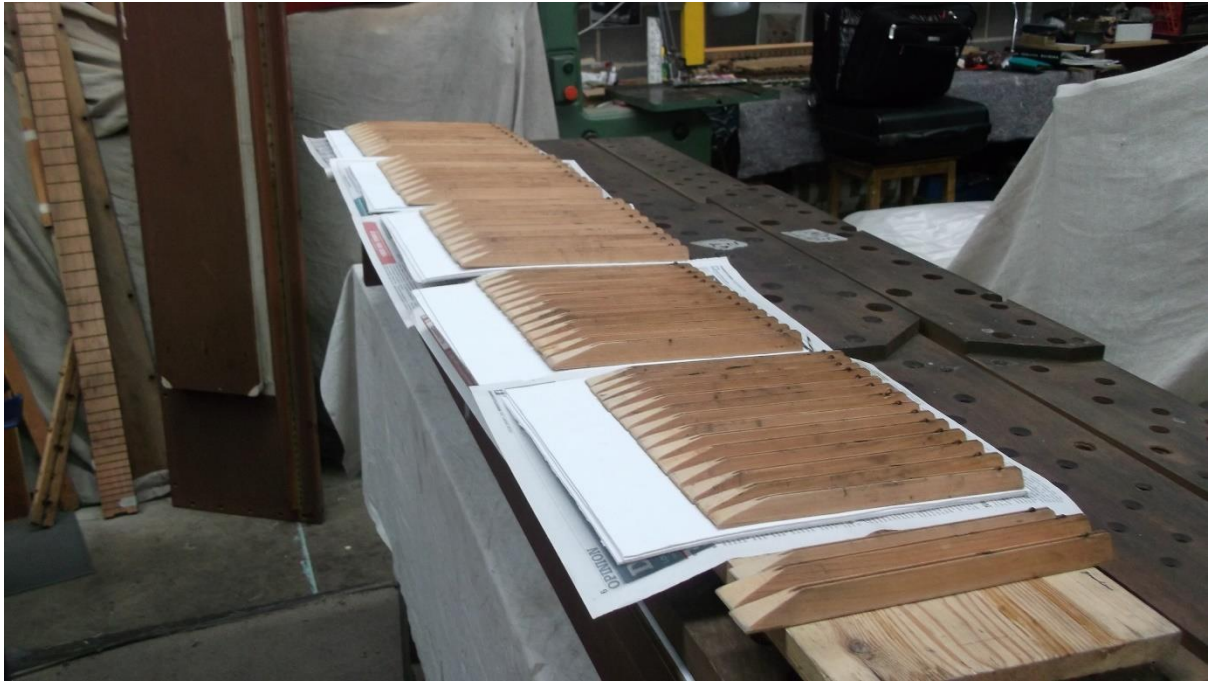
The pallets of both Swell and Great with new 3 ply leather coverings.
