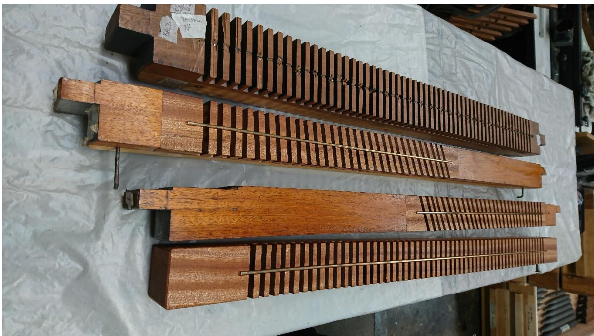
The action beams remade with hard-wood sections.
