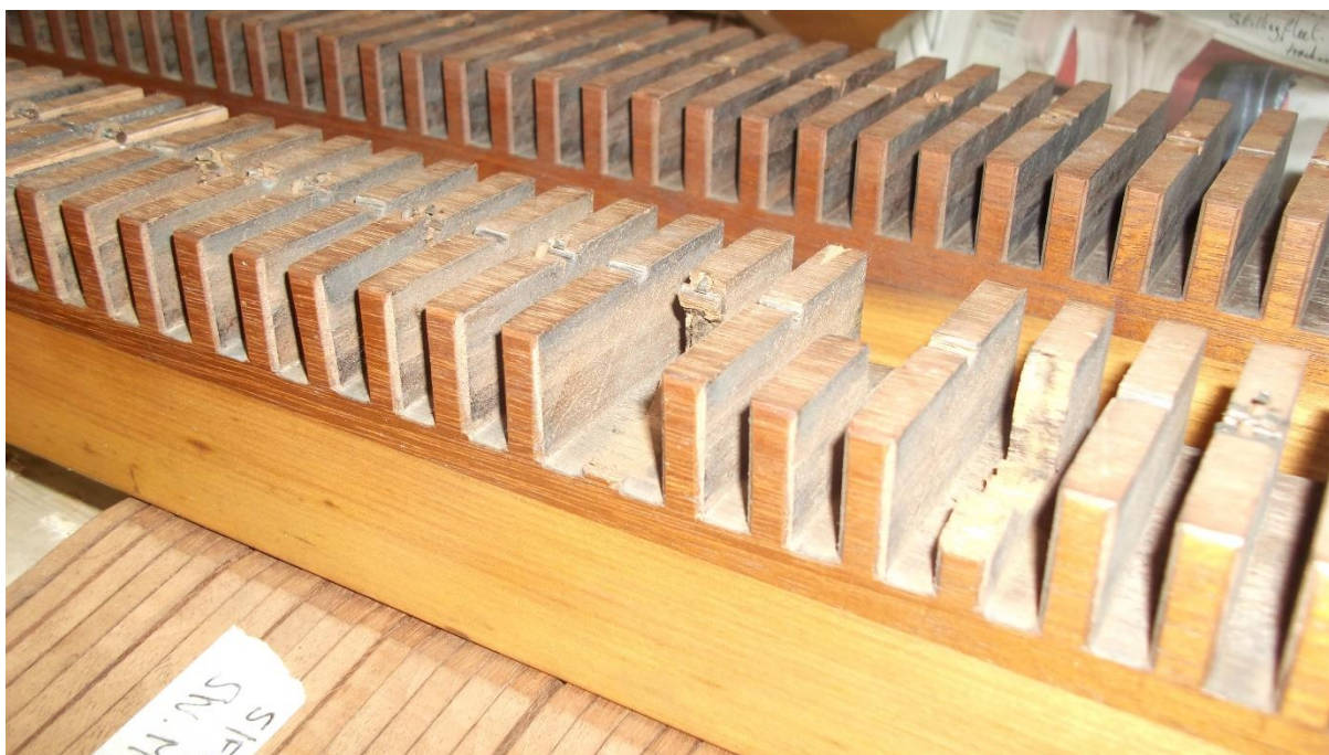
One of several of the backfall beams with the split and missing sections.
