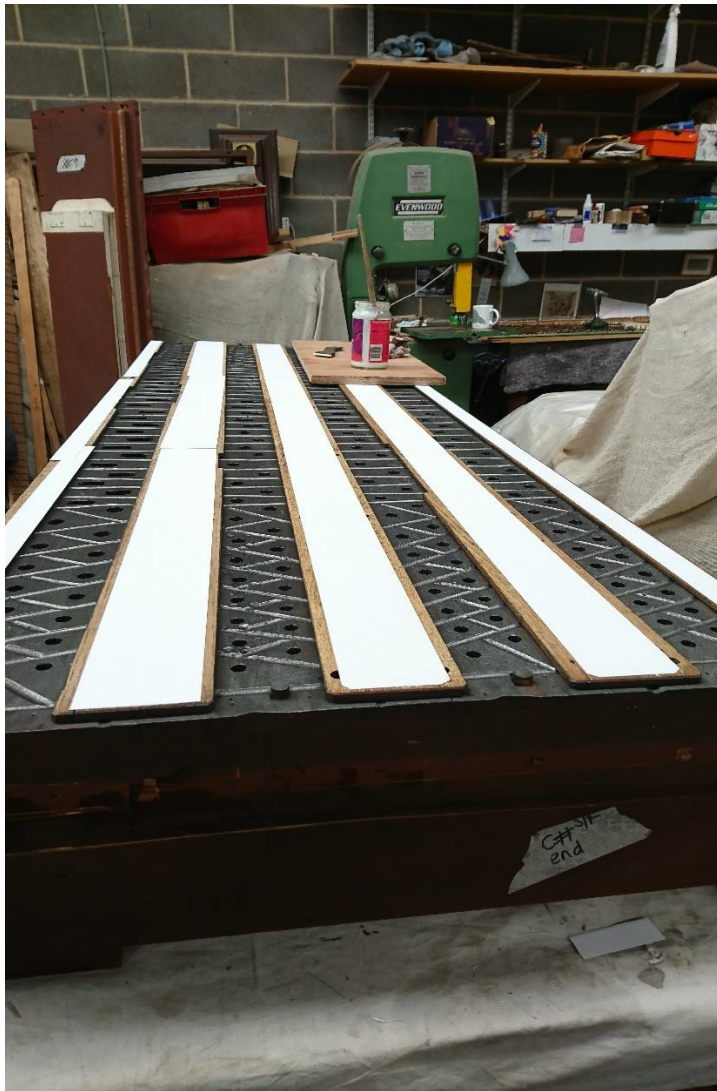
The Swell soundboard with table top planed and bearers papered ready for the sliders and upper-boards.
