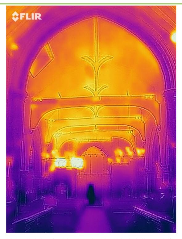
This image clearly shows that the heat rises to the ceiling. The heating had been running for approximately one hour.
