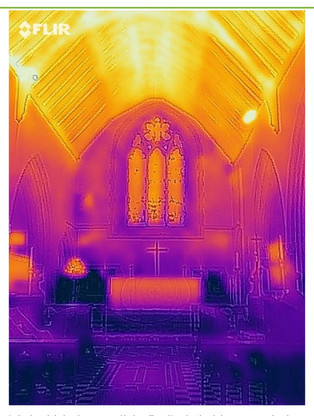
In the chancel, the heat is concentrated in the ceiling. Note that the windows are warmer than the surrounding stonework (it is normally the other way around). This is due to the external polycarbonate covers.
