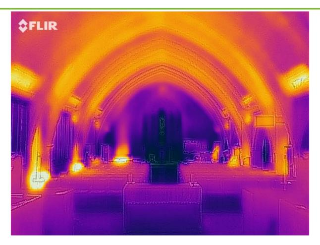
Actual temperatures, measured using an infrared thermometer were: Tiled floor 16.2, Carpet 17.7, South wall 17.3, West wall (away from heaters) 15.0, font 16.2 (a good indicator of the temperature of a church and how much the building is used due to its large thermal mass), ceiling 20.1 (three degrees warmer), heater case 66, element inside 200.
