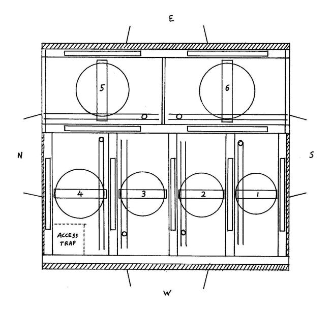
Note. The cross-hatched areas indicate the position of masonry infilling between the support grillage and the tower walls.
