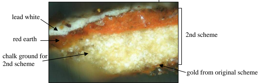
Photomicrograph of sample 12 x200 Normal light
